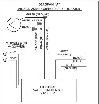
Figure 2-1: Connection Wiring Directly to Central Heating Circulator
